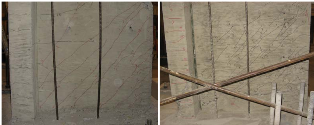
Figure 5.2. Structural-wall crack patterns near end of test (left: conventional concrete, right: HPFRC)
